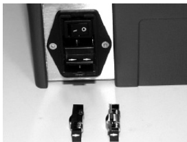
Carefully remove fuses.
