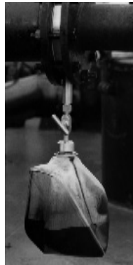
Sampler in use on a Bunker Barge.
