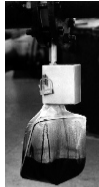
Sampler with valve lock fitted to satisfy PSA guidelines.
